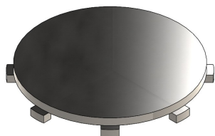
10.0 x 1.0 ½" Plate with ½" Lugs Perimeter Gap Class E
